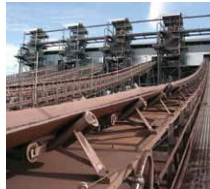
Photos 43 –46: The Sishen expansion project including some 22 000 tons of hot dip galvanizing in the form of process and conveyor steelwork.
