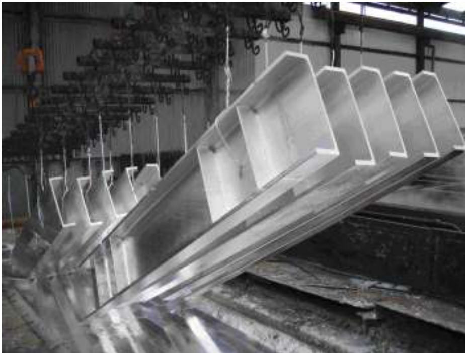
Web forged steel channel products being hot dip galvanized
