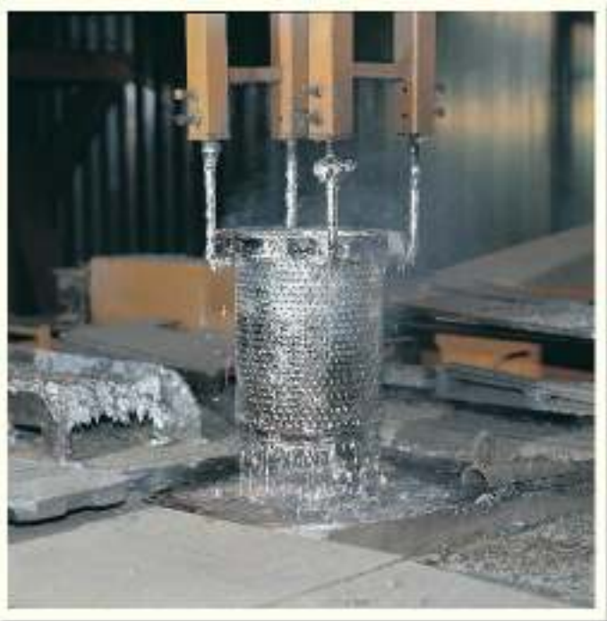
Spin hot dip galvanizing of small components such as nuts, bolts, hinges & fixtures
